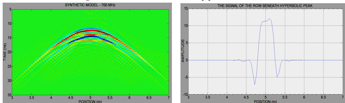
Fig. 2a: GPR section of the model 1
