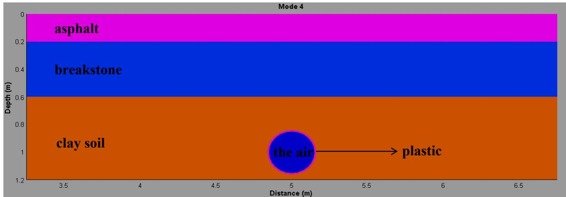
Fig. 5: Vertical section of the buried pipe in model 4
