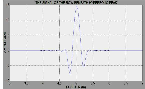
**Fig. 4b: The signal of the row beneath hyperbolic peak**
