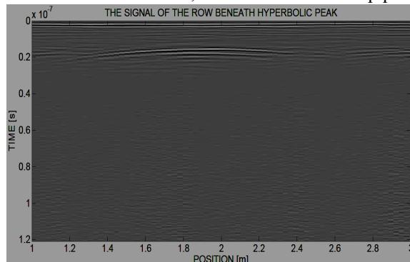
**Fig. 7a: GPR section of the water supply pipe data**
