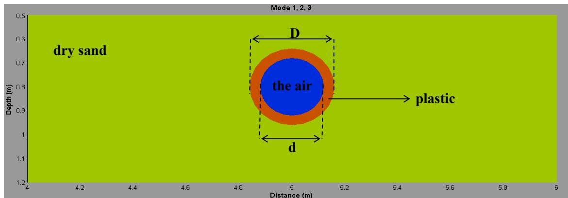
Fig. 1: Vertical section of the buried pipe in model 1, 2, 3
